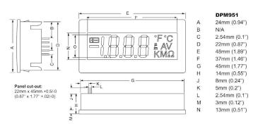
36mm x 72mm (1.4in x 2.8in) Panel mount digital meter with a 200mv full scale input. 14mm height character display with annunciators for common engineering units and suitable for operation with either 5VDC or 9VDC power.
