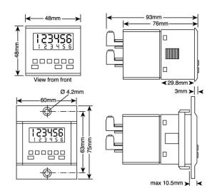
6 digit supertwist LCD programmable preset counter with prescaler, quadrature input and EEPROM data storage in an IP65 (NEMA4X) DIN case.
